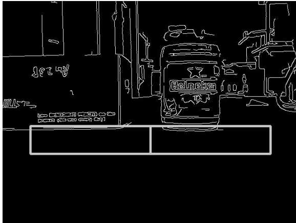
Fig. 5. Obstacle Detection Regions
